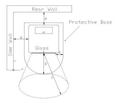
While installing the stove, the fire regulations and chimney's instructions must be complied. For any related questions please ask the chimney installer. Minimum distances to be observed in flammable or heat-sensitive materials (eg furniture, wallpaper, wood panels) (see diagram below) are:
